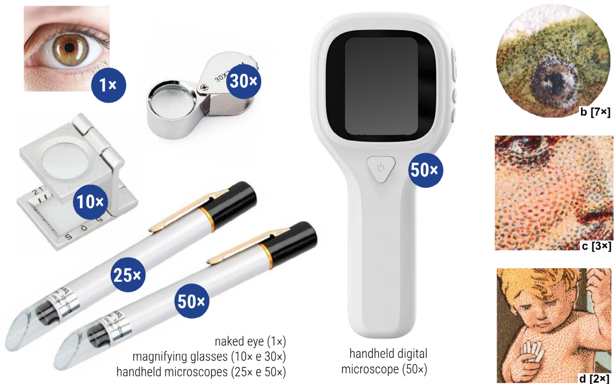
Figure 2 Visual assessment, magnifying devices, and digital microscope used for analyzing the microstructure of printed materials, with examples. Source: Barros, 2018, updated, 2025.
